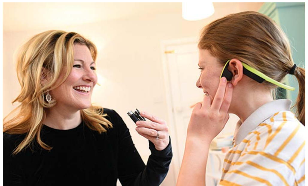
Figure 3. The bone conduction headset can be paired to a microphone, which may be held by a parent or teacher
